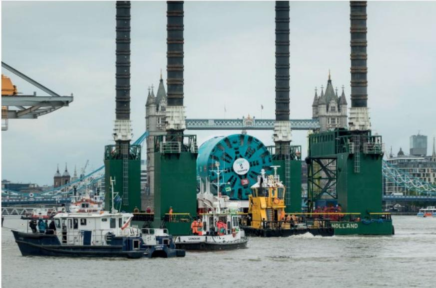
A tunnel breaking machine being transported by river to the Thames Tideway Project. *Thames Tideway Tunnel*
